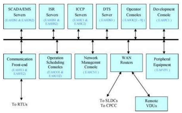
The equipment Ids are marked as blue in the above mentioned diagram. The details of networking equipments and printers / loggers are not included.
